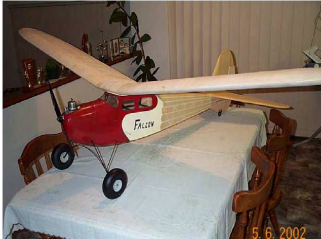
Falcon Old Timer – 8 foot wingspan and Merco 35 diesel
